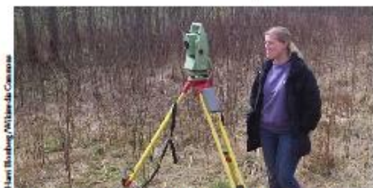
Archaeological survey using a Total Station on an Iron Age dwelling at Ytterby, Sweden
